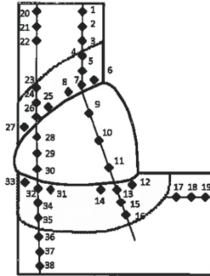
Figure 7 Locations of Hardness Survey Indents for a Set-on Branch Fitting.
