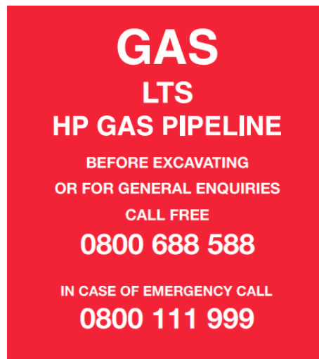
Figure 8: Example format for aerial marker post adhesive notices for Gas Distribution HP pipelines
