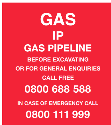
Figure 9: Example format for aerial marker post adhesive notices for Gas Distribution IP pipelines
