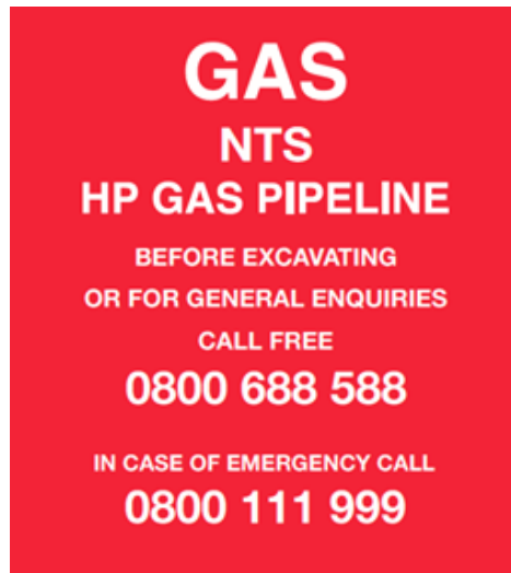
Figure 7: Example format for aerial marker post adhesive notices for Gas Transmission (NTS)
