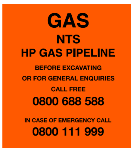
Figure 10: Example Face Plate for M4 HDPE Field Boundary Marker Post for Gas Transmission (NTS)
