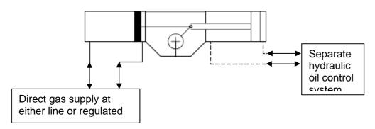
This method only applies direct gas pressure onto the pneumatic cylinder side of the actuator to stroke the actuator. This method of operation is used during normal modes of operation. However there is a separate hydraulic manual override control system that will, in the event of gas pressure being lost, provide an alternative method of stroking the actuator.
