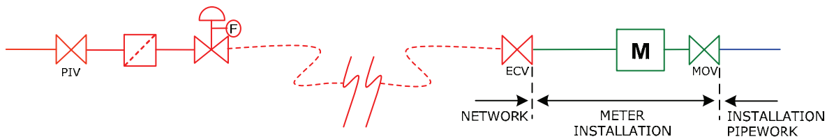
FIGURE 37 - LEGACY ARRANGEMENT 75 mbar < SUPPLY MOP ≤ 7 bar REMOTE SERVICE REGULATOR AND NO METER REGULATOR CAPACITY > 6 m 3 h -1
