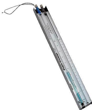
*Fig 1. Manometer “Water gauge”*
